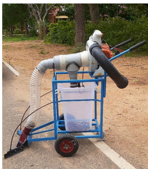
Fig. 5(a). Ground collection machine for Neem fruit.
