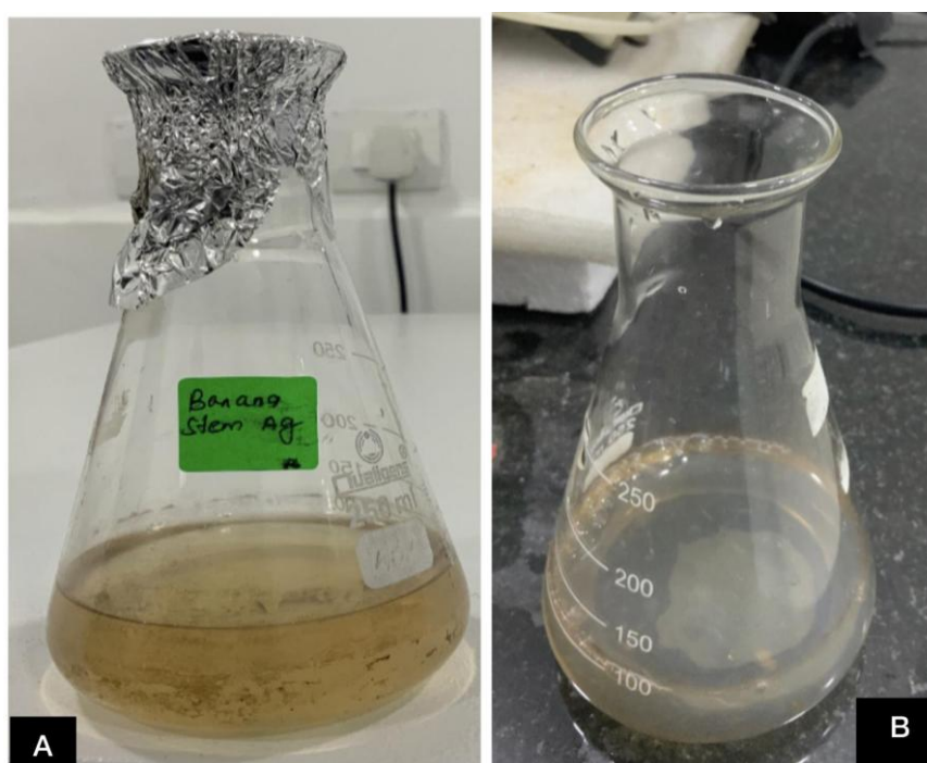
Fig. 2. Image showing the preparation of Musa sapientum mediated silver nanoparticles. A - Musa sapientum extract. B - Silver nanoparticles solution
