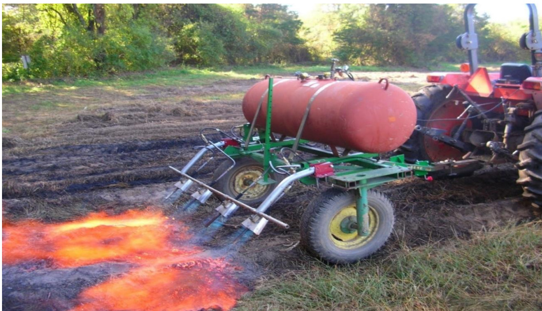
Fig. 6. Flaming weed control using propane gas
