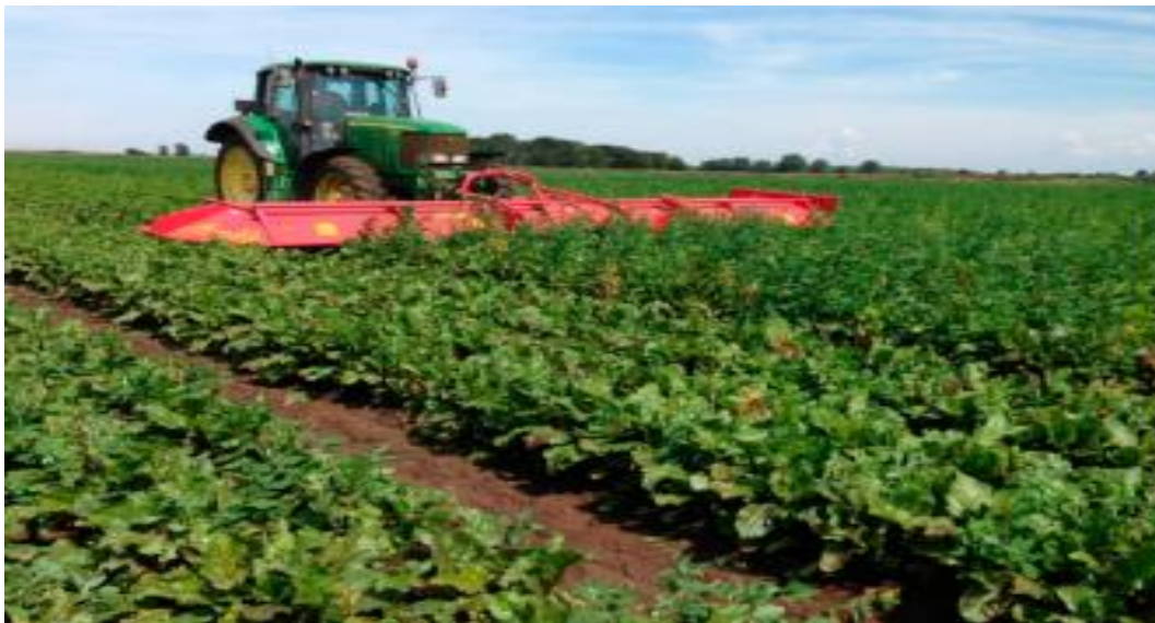
Fig. 2. A weed header (weed surfer) in action surmount weed seed heads come through above an organic organic beetroot ( Beta vulgaris L.) crop (Photo: S Briggs). beetroot ( Beta vulgaris L.) crop (Photo: S Briggs)
